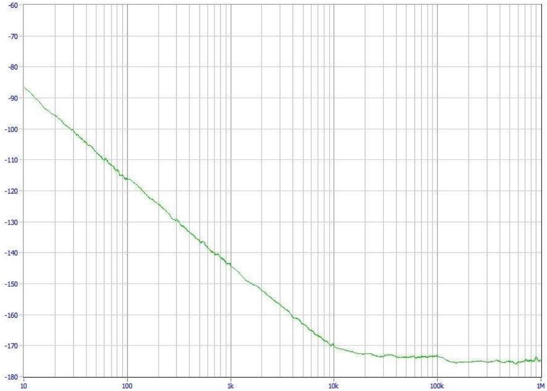
Typical Phase Noise at 100 MHz
